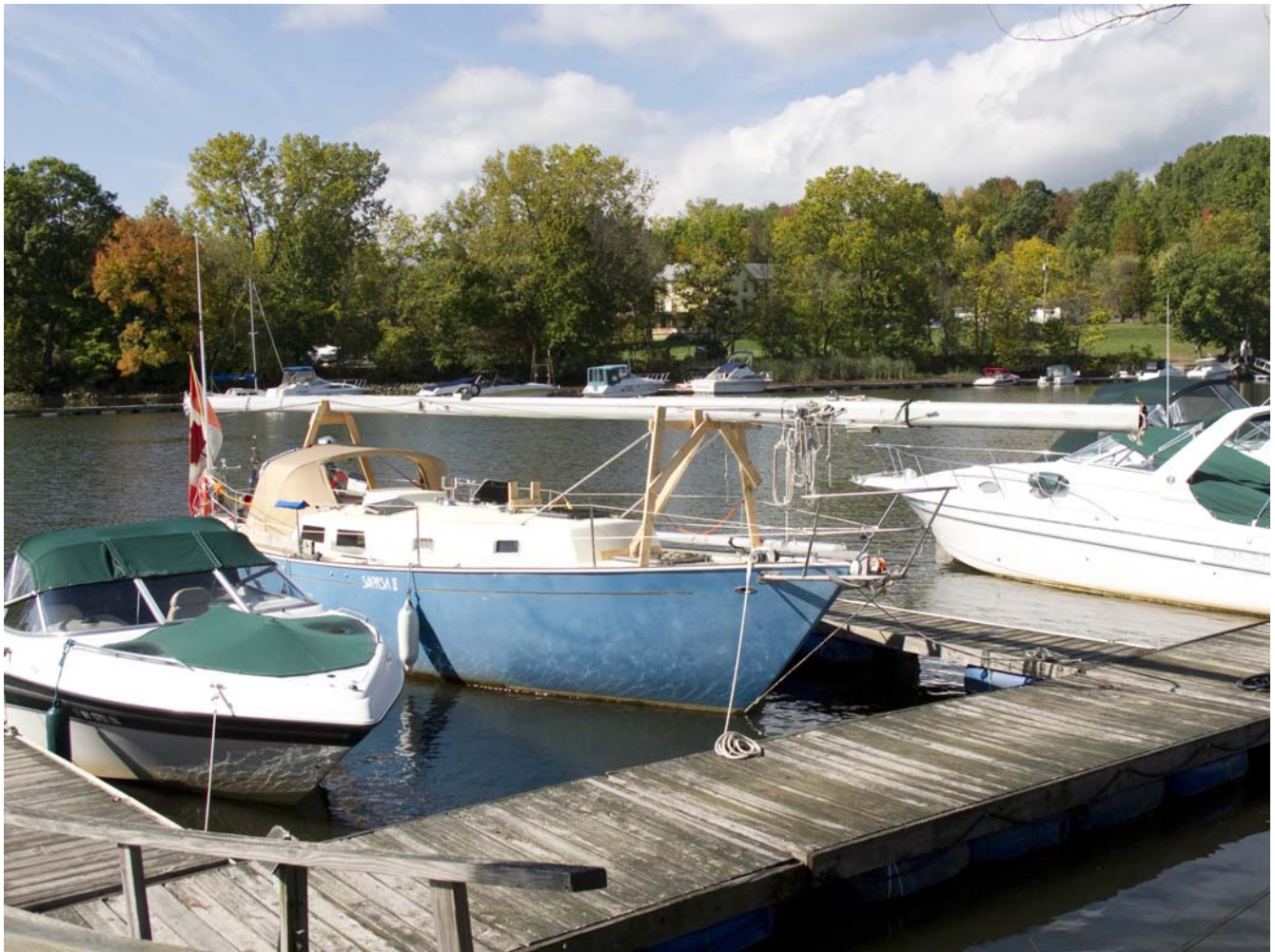
Illustration 42: At Catskill, mast unstepped and stowed on deck ready for Erie Canal transit
